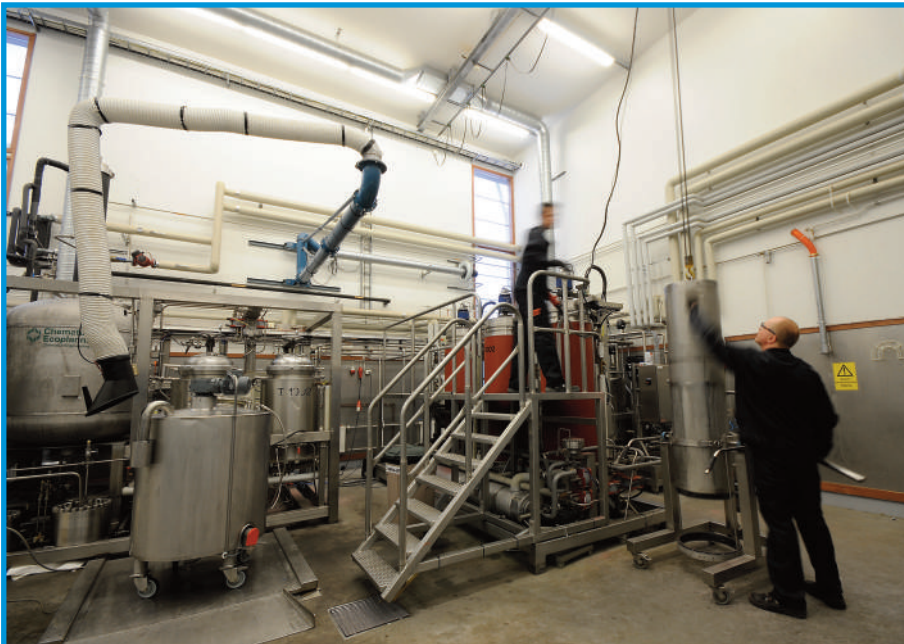
Supercritical CO 2 -extraction at Aromtech Ltd in Tornio, Finland. Facility is registered for processing foods including organically certified materials
